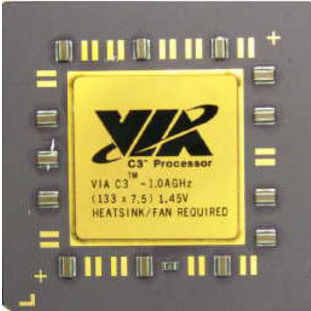
Picture of the VIA C3 low power 1.0 GHz CPU.
